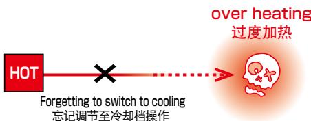
It is necessary to switch to cooling operation to cool down the heater after heating. If you forget to switch to cooling operation, the internal parts may be damaged or the heater life may be reduced due to the overheating.
