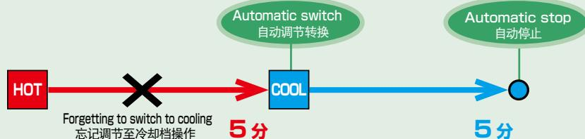
Even if you forget to switch to cooling operation, this unit automatically switches to the cooling operation 5 minutes after the heating operation started to prevent overheating problems.
